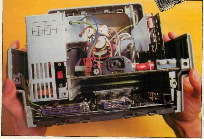
Taking a closer look at the Model 16 reveals signs of this intended role. The various components of the system are connected together in a neat way with cables that terminate in a standard connecting block. Each block has a plug on one side and a socket on the other, so you can push another block into the back of it, letting you piggyback several cables into the one HPIB socket on the back of the main unit.
